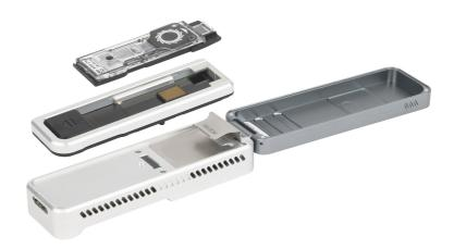
The Flongle adapter contains 126 channels. Each nanopore channel is controlled and measured individually by the bespoke ASIC. This allows for multiple nanopores to be run in parallel. Users can simply insert Flongle flow cells into the adapter, run their experiment and then discard the Flongle flow cell and replace it with another.
